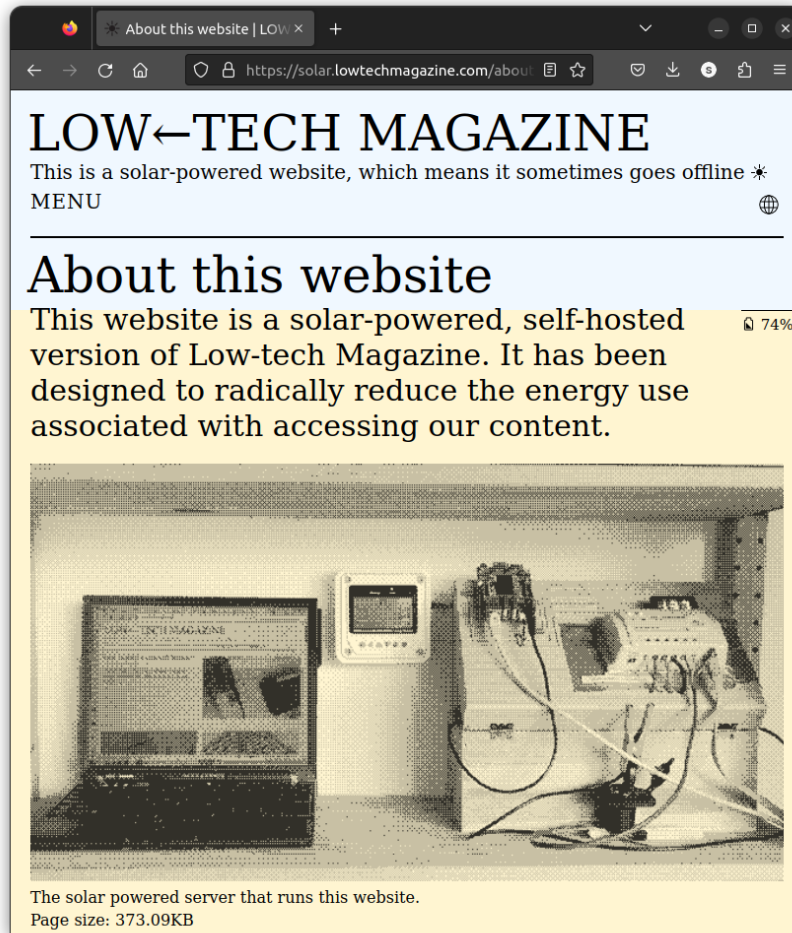
Figure 2.1: About this website - Low-Tech Magazine. The background color indicates the current SoC, the image used is dithered but still reasonably recognizable, overall resulting in a page size of only 373 kB.
